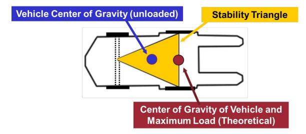
Keeping the downward force of the load (center of gravity) within the stability triangle keeps the forklift stable and keeps the load from crashing to the ground. Allowing the load to move outside the stability triangle makes both the forklift and the load less stable and subject to tipping, rolling, or dropping.
