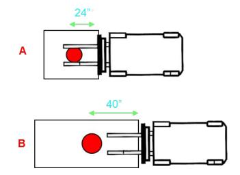
So understanding the center of gravity and load center helps the operator to determine how to pick up a load and maintain stability (pick up the load on the side closest to the center of gravity). In example B above, the load should be picked up from the side, not the end, as shown.
