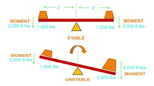
From that bit of knowledge, let's define a couple of more terms that will help us determine the stability of a forklift. Earlier, we mentioned the center of gravity and load center. The center of gravity is the average location of the weight of an object. The load center is the distance from the carriage, or vertical face of the forks, to the center of gravity of the load.
