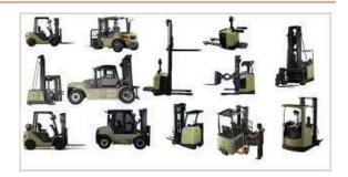
All forklifts have some things in common. They have forks that pick up the load, hold it during transit, and put it in place at the new location. Forks tilt forward or backward. The operator can adjust the space between forks to lift loads of varying widths. Some forks on forklifts can be replaced with special attachments for carrying oddly shaped loads, such as drums, or long loads, such as pipe. Some can be used with a manbasket for elevating people.
