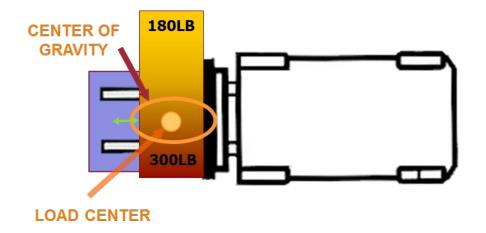
If a load contains materials with different weights or densities, the center of gravity will be on the side containing the heavy material. For example, if a pallet contains bricks on one side and feathers on the other, the center of gravity will be closer to the side of the pallet containing the bricks.
